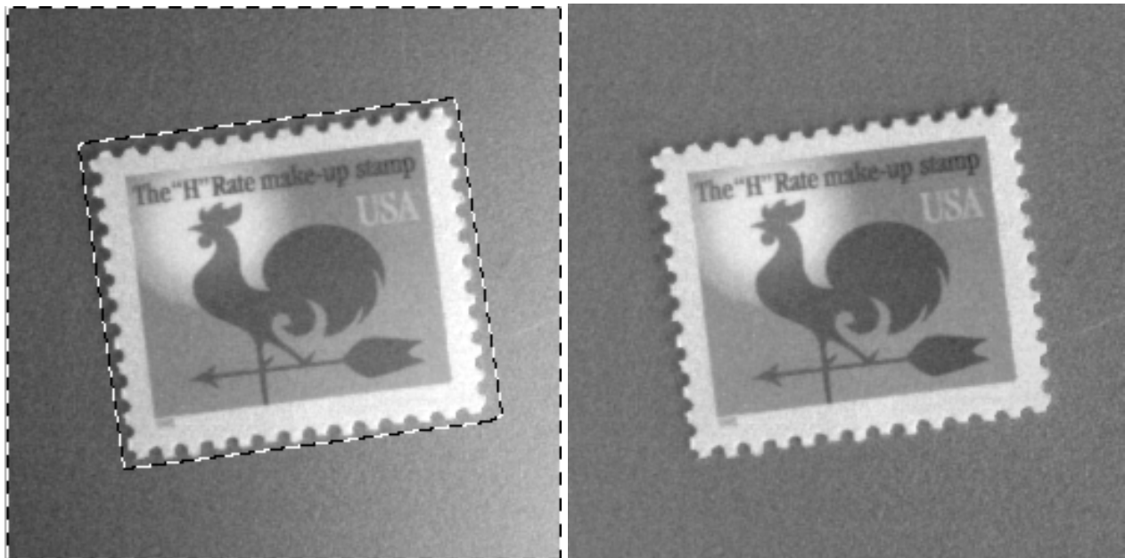
Fitting and subtracting a background function to a selected region.
