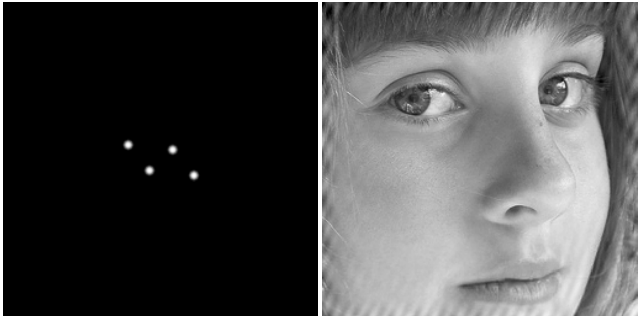
Noise removal filter and resulting image.
