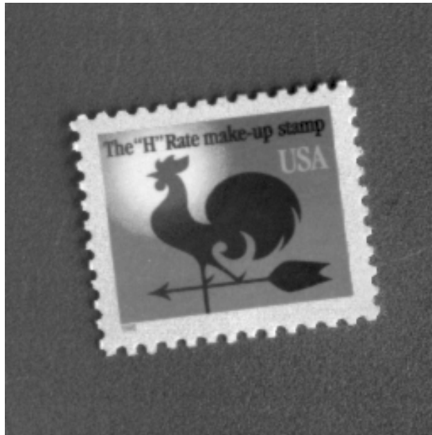
Subtracting the background image produces a result with uniform lighting.
