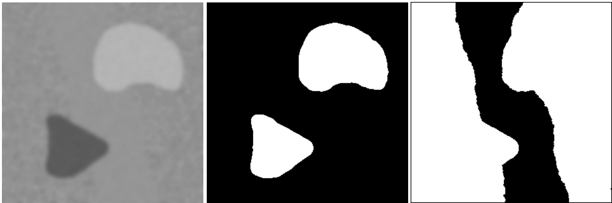
Gaussian blur applied; medium grey region thresholded; Boolean AND NOT used to combine thresholded binary images to select just the smooth, medium brightness region.
