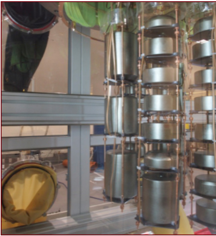
Figure 2: Germanium detector strings used in the Majorana Demonstrator to search for neutrinoless double beta decay.
